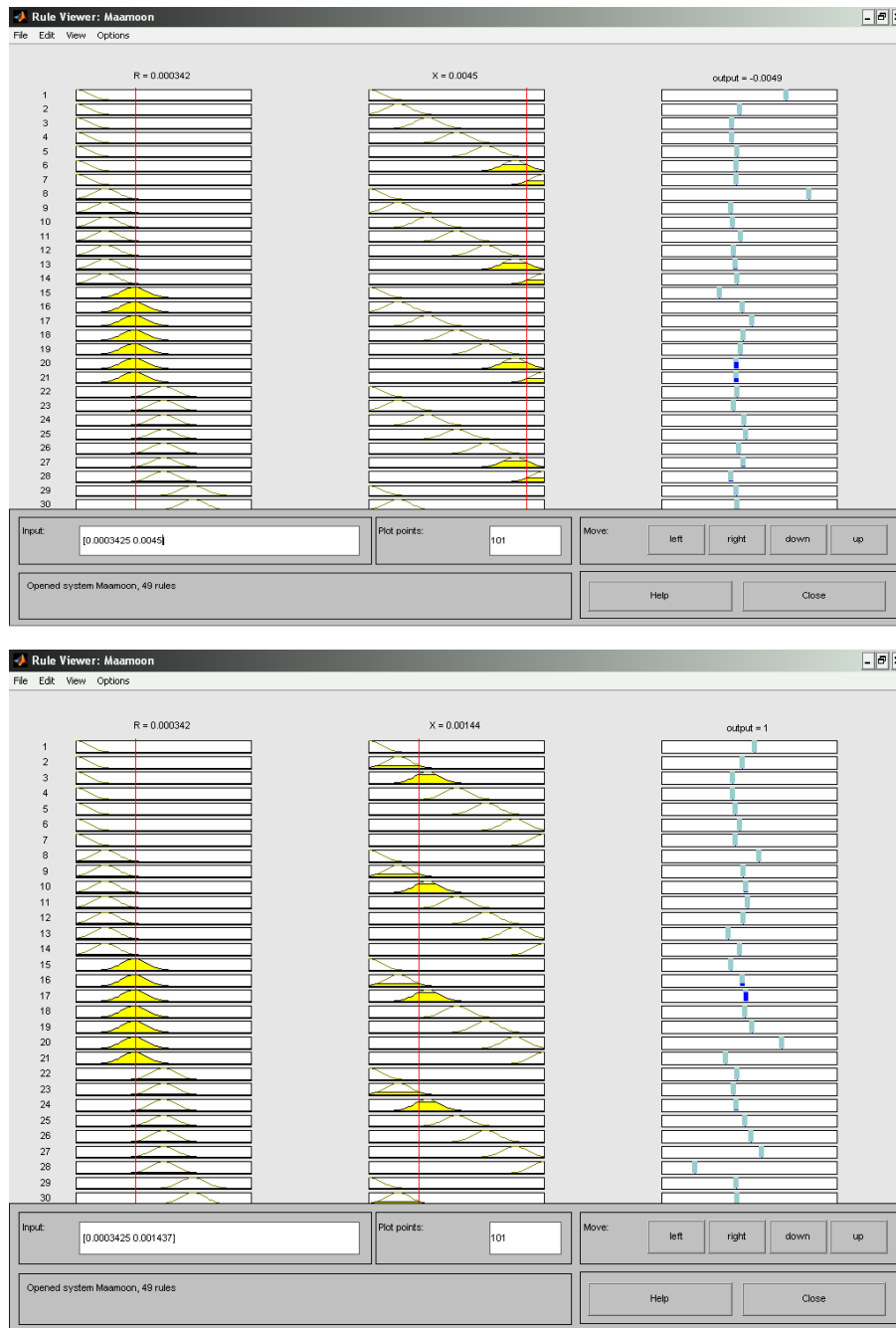
Figure (10) Test results of membership function & Sugeno corresponding response.
